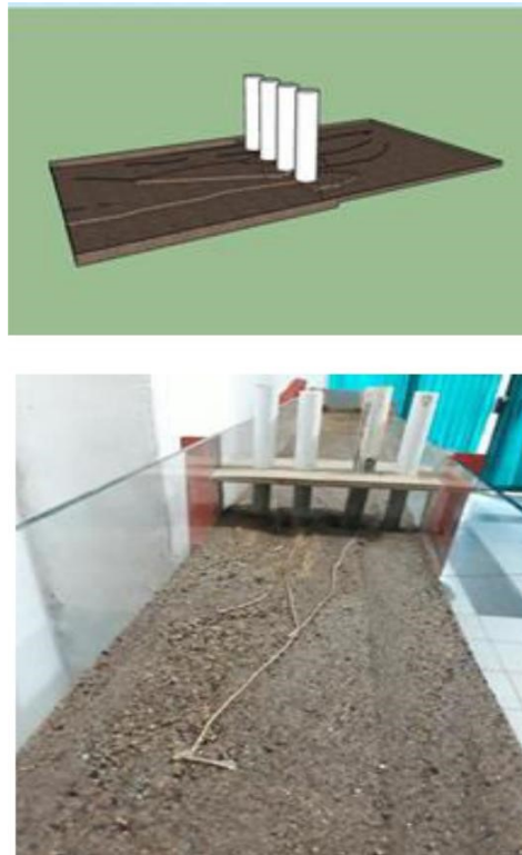
Figure 10. Sediment movement pattern during t = 30 '.
